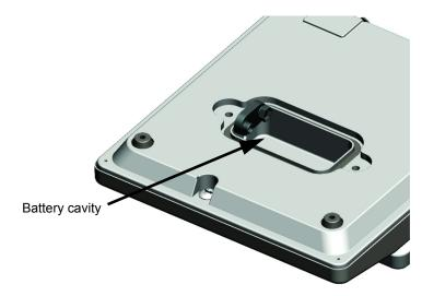
3. Install the 9V alkaline battery
