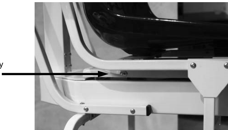
Figure 12. These Screws Hold The Molded Chair to the Scale Base
