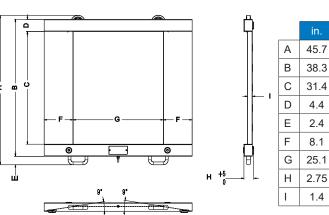
Portable: Fitted with two handles and wheels to easily relocate
