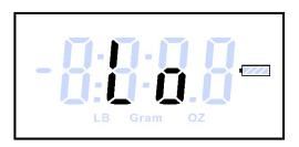
In this case, the user will also see the empty battery icon blinking and once it appears, the user should immediately replace the battery as the low battery condition is likely to degrade the weight measurement and giving a poor accuracy.
