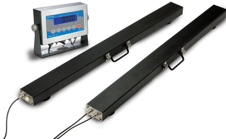
The WB-521 Series Weigh Beams are pre-calibrated with the SBI-521 LCD Indicator. This highly portable scale system is designed with simplicity in mind. In just a few minutes, the entire scale is set-up and ready to weigh. The Weigh Beams have built-in handles and 4 m / 13' of load cell cable with quick connectors. Each beam is only 16.5 kg / 36 lb light enough to be carried by one person.
