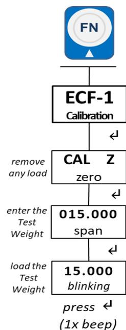
*Before starting, make sure that LF 3 and LF 7 are configured as desired and test weight equivalent to at least 1/3 of the maximum capacity.*
