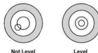
**!** *Always check the level prior to using scale.*
