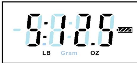
If users require the result in metric or decimal LB units, press the selection key once and the readout will toggle to metric 2622 gram
