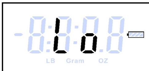
In this case, the user will also see the empty battery icon blinking and once it appears, the user should immediately replace the battery as the low battery condition is likely to degrade the weight measurement and giving a poor accuracy.
