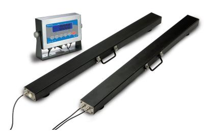
The WB-521 Series Weigh Beams are pre-calibrated with the SBI-521 LCD Indicator. This highly portable scale system is designed with simplicity in mind. In just a few minutes, the entire scale is set-up and ready to weigh. The Weigh Beams have built-in handles and 4 m / 13' of load cell cable with quick connectors. Each beam is only 16.5 kg /36 lb light enough to be carried by one person.
