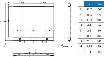
**Ramp:** Designed with built-in 9 degree gradual angle to make entry and exit safe and easy
