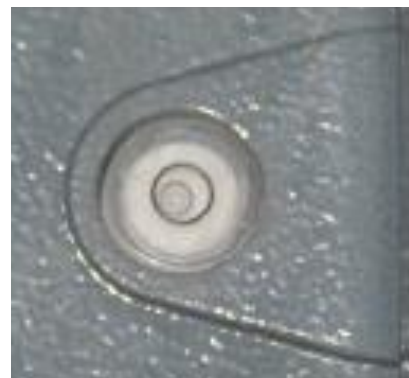
Fig. 2 Adjust feet until bubble is centered in black circle
