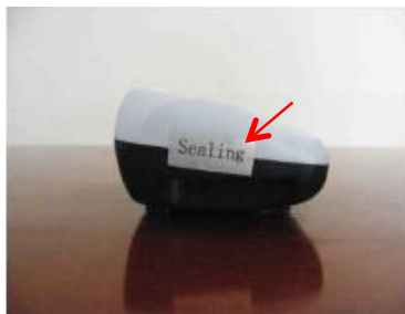
Sealing with supplied tamper proof labels
