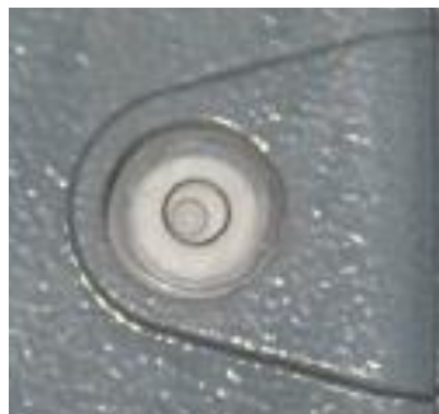
Fig. 2 Adjust feet until bubble is centered in black circle
